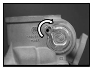
Install the M5 screw without tightening it.
