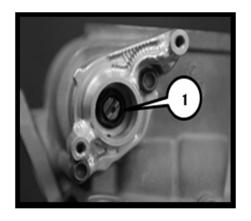
Remove the two M5 screws [2] from the valve motor bracket and remove the bracket from the cylinder.
