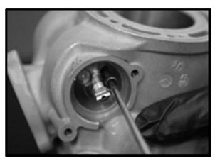
Fit back the setting washers on the valve shaft.
