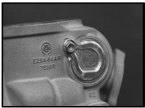
Fit the connecting screw of the half-valves and tighten to 6 Nm.
